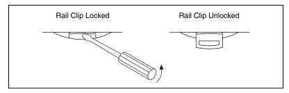
Figure 2-1. DIN Rail Clip
